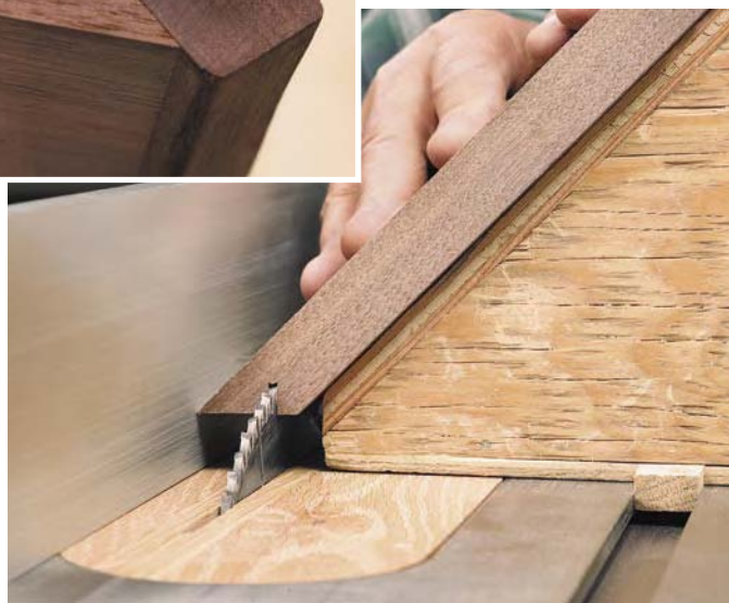
Each mitered end of the aprons receives a slot for the splines. The completed joint is strong, even though the splines are thin (inset).
