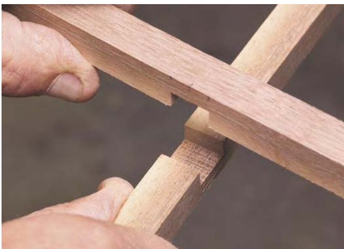
A bridle joint holds the stretchers together in the middle, dowels join the ends of the stretchers to the legs.
