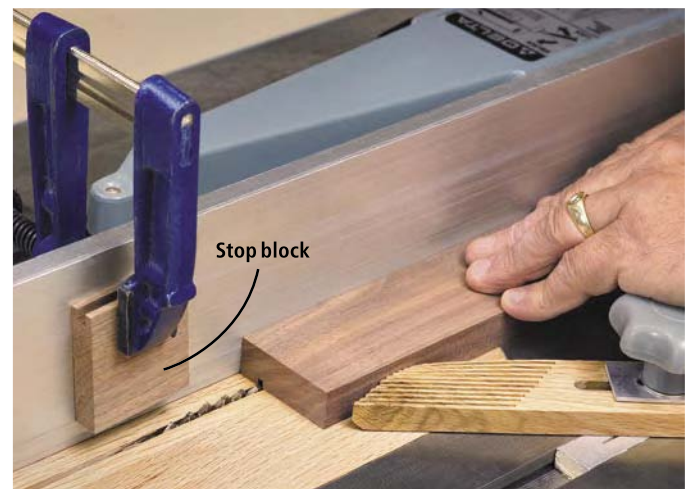
A stopped groove is cut on each side of the legs for the splines that will join them to the aprons. A stop block ensures accuracy.
