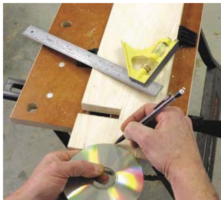
One simple joint is all it takes to build these shelves. The decorative cut is laid out by tracing the edge of a CD.
