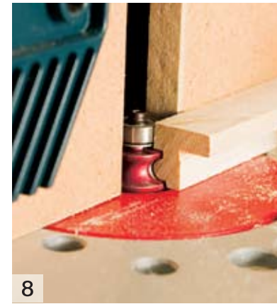
We milled the inside trim molding. Cut the molding profiles on the router table using a straight bit to cut the rabbet and a 1/8-in.-radius edge-beading bit to cut the edge bead.
