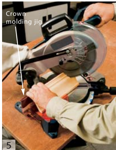
When cutting the side crown molding pieces, first make the 45-degree miter cut in a longer piece. (For additional safety and accuracy, we also used a jig that holds the molding in position.) Then cut the mitered crown molding to length.
