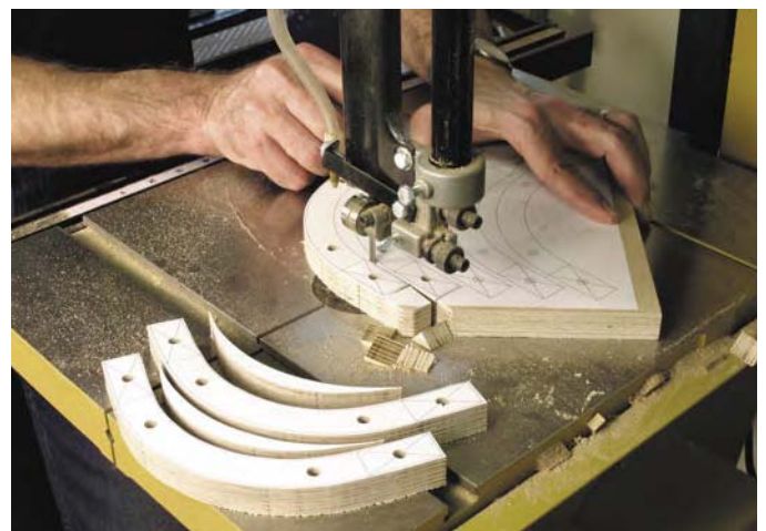
Nesting the patterns for the corner segments produces a minimum amount of waste. Make the cuts just outside the lines. You'll be a band saw master by the time you get to your 36th smiley.
