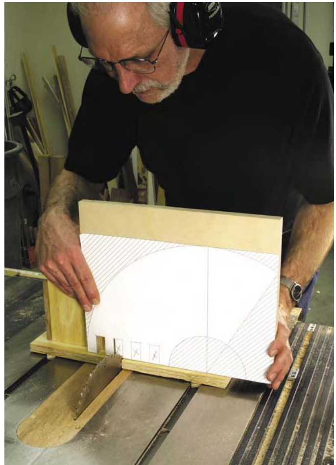
My dado sled is nothing more than a scrap of plywood fastened to a couple wood runners. The fence is mounted square to the table and perpendicular to the blade. Here, I'm removing the finger-joint waste from a tabletop half.
