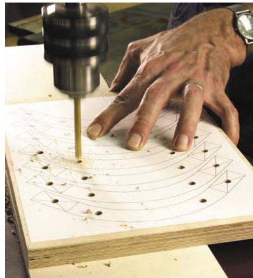
This obligatory "Man Drills Holes In Board" shot is here to remind you that accurate drilling, with a backup scrap to prevent tear-out, is key to a number of forming and glue-up steps. A 17/64 " brad-point bit clears the way for the 1/4 " registration dowels.
