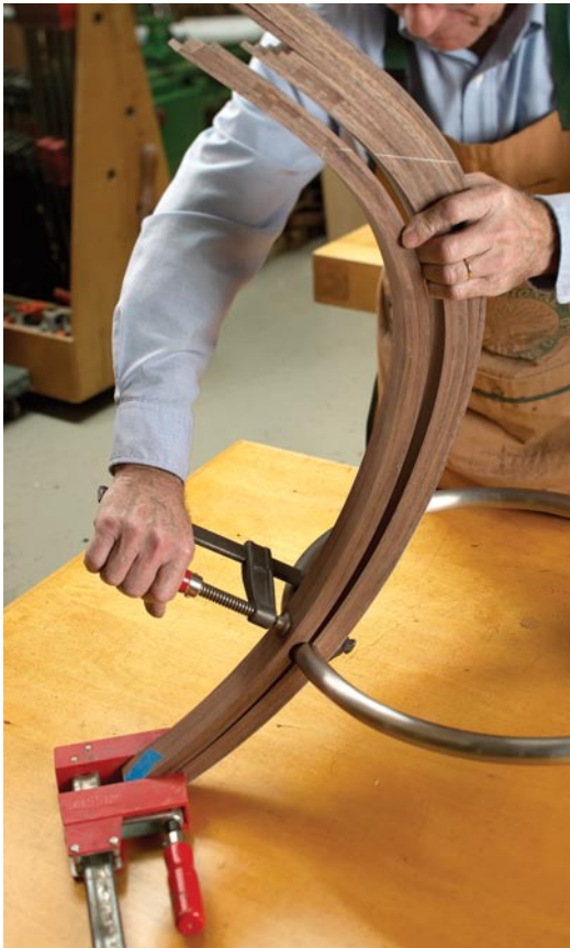
No hardware needed. The stainless steel rail pierces the finished legs. The two halves were clamped together to drill the holes.
