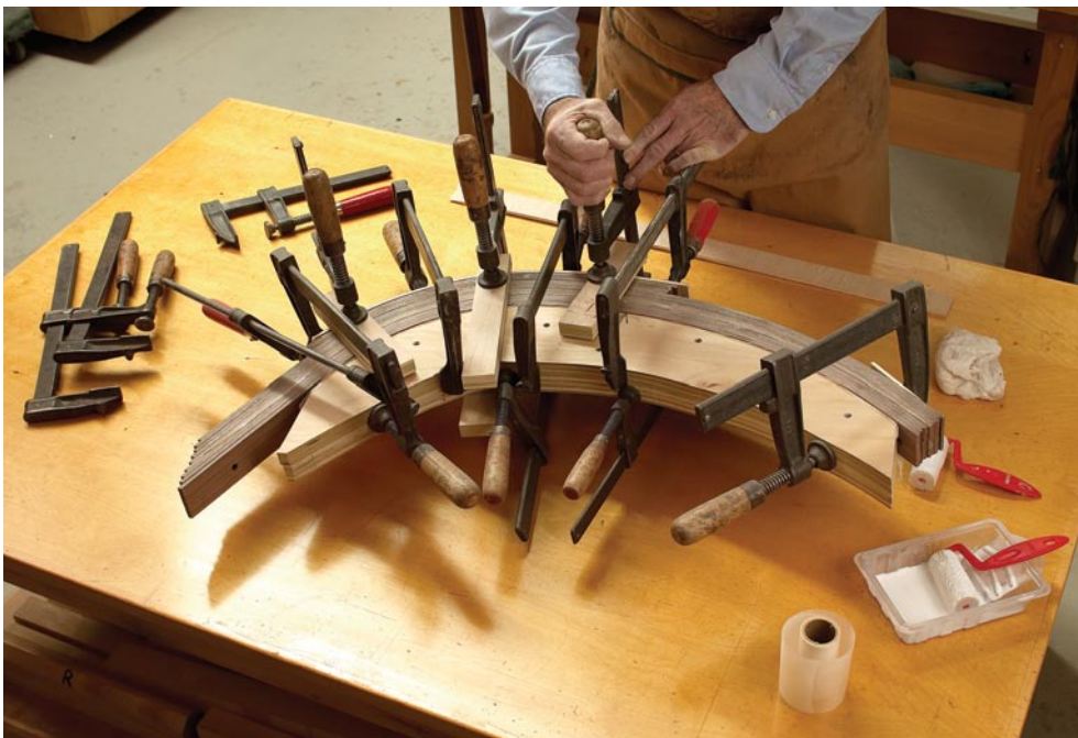
Curves with a twist. The strips are glued to a plywood form. To allow the steel ring to pass through the legs, they are glued as two halves.
