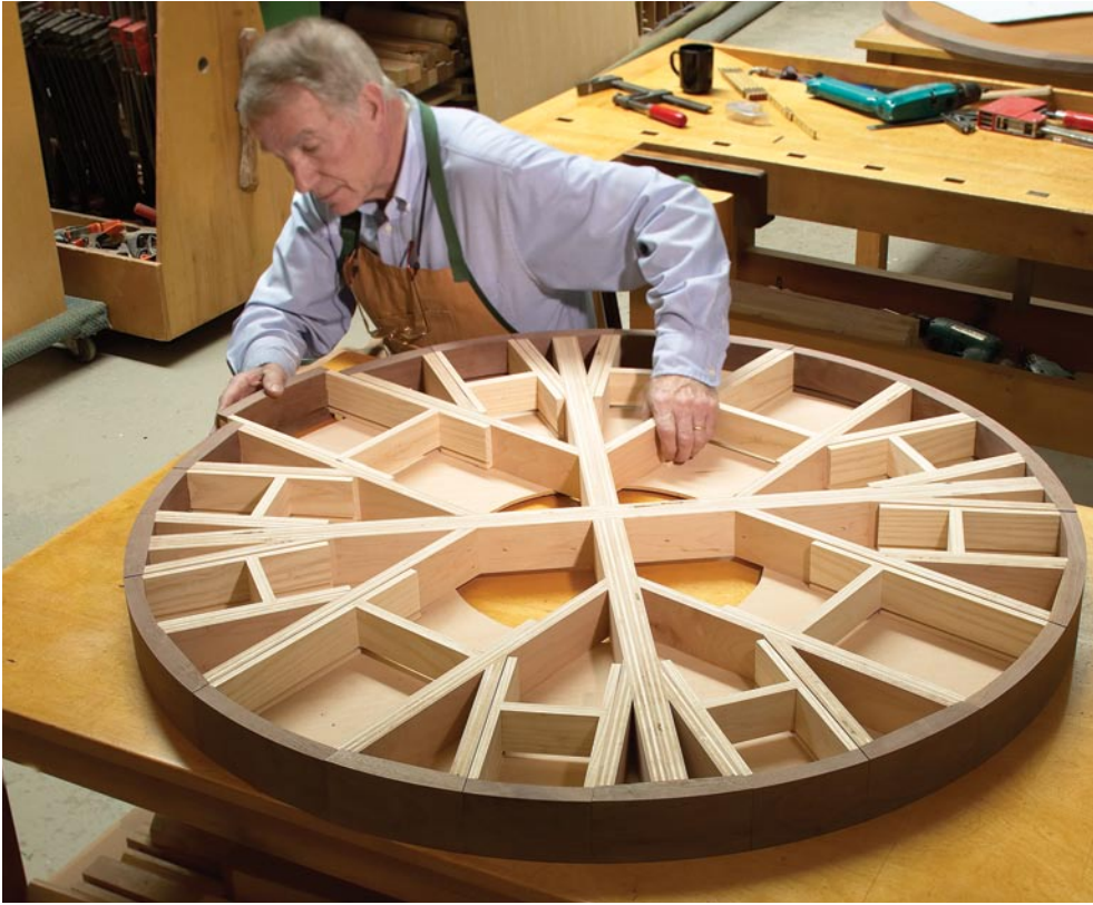
Solid-sawn aprons and trim. All of the solid-wood parts of the apron were band sawn and fit into place before final shaping.
