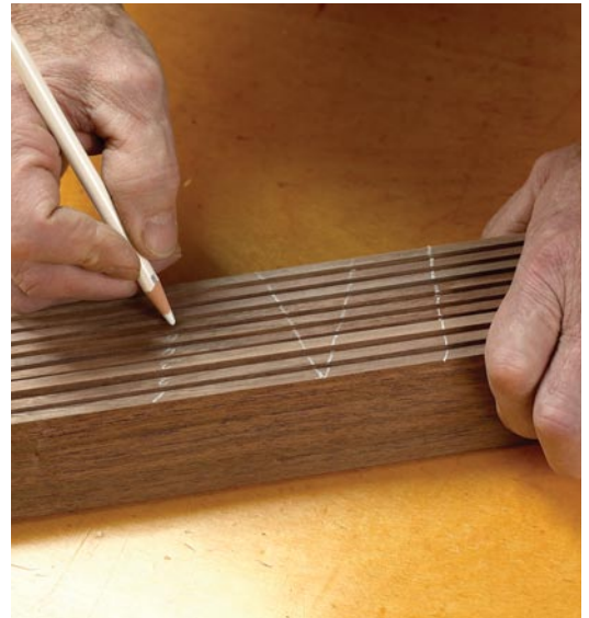
Preserving the grain. A triangle made with a white pencil helps keep the strips in order. When glued together they will look like a solid piece.
