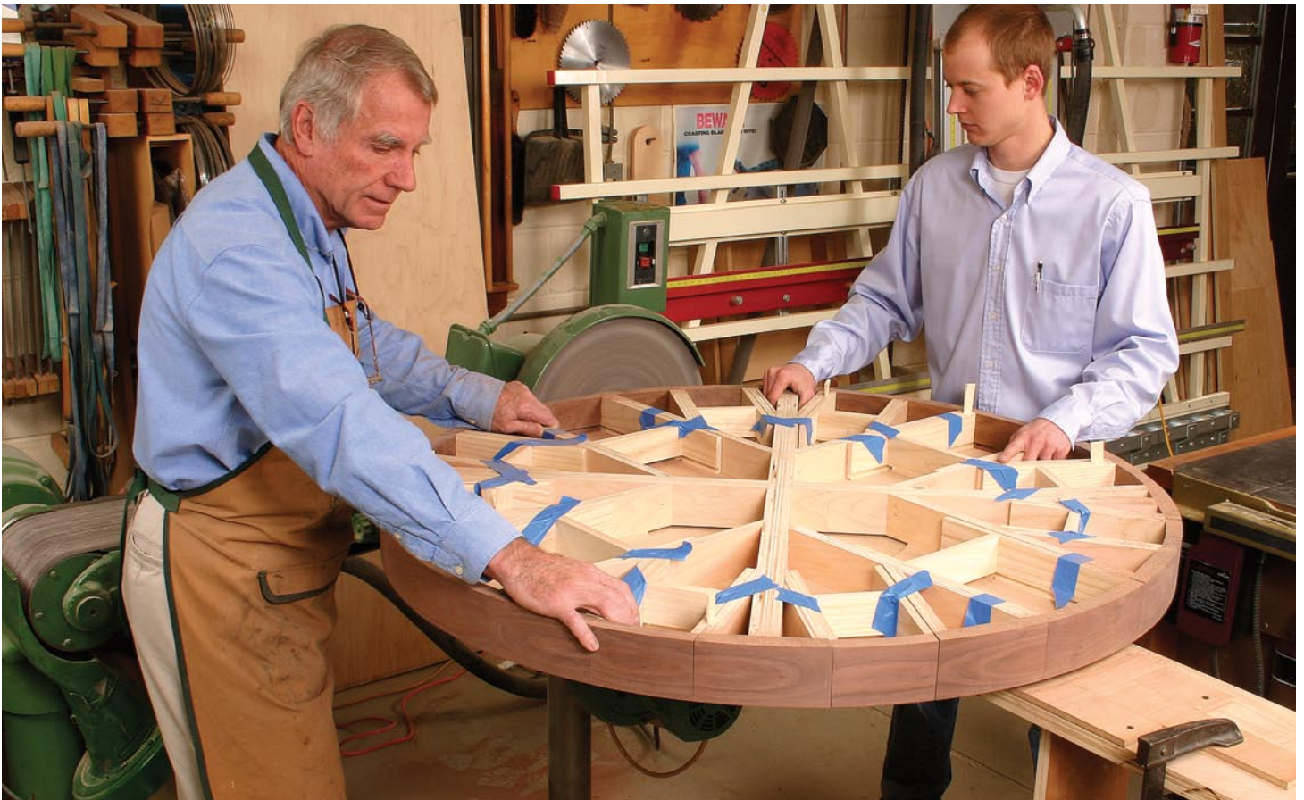
Round and round. Klausz and Douglas Bloom shape the drawer fronts and apron to a perfect circle with a trammel set up on the disc sander.
