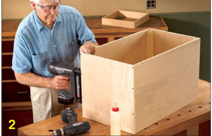
Assemble the boxes with glue and 1-1/4-in. screws. Attach the corner blocks to the main box with glue and 1-1/4-in. brad nails.
