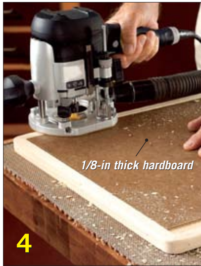
Use a router and 3/16-in. roundover bit to profile the lid edges. A scrap of 1/8-in.-thick hardboard keeps the router base level.
