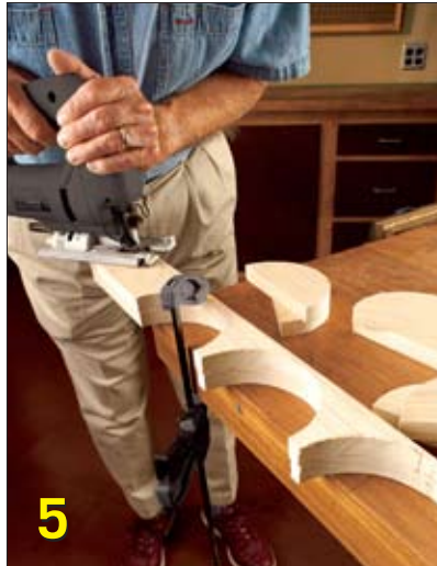
Gang cut the wheel halves with a jigsaw. Cut just outside the line and then sand back to the line.
