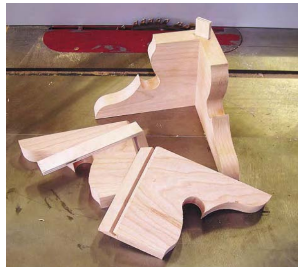
Remember when making the 45° cut for the splines that you need to adjust the blade height as well. Then make the splines that will fit into the slots and glue the front feet together.
