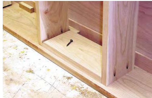
Using pocket hole screws to attach the shelves allows you to remove the shelves to make finishing easier.
