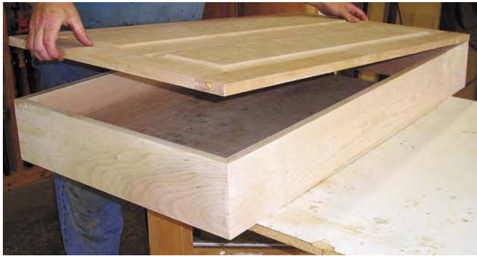
Glue the door panel to the door frame, allowing an even overhang on all sides. Check the door for square after glue-up.
